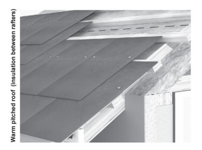
Where Permavent Vapour Permeable underlays (type LR) are used in both cold and warm roofs to contribute to the control of condensation, they do so by allowing water vapour to escape through the material by diffusion. It is important that this water vapour can escape to atmosphere from the batten space. BS 5250 defines a test to determine whether a roof covering is sufficiently air open and asks manufacturers of the roof covering to provide advice.
